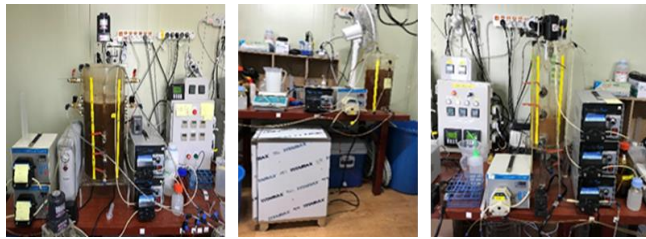
Fig. 1 Lab-scale AGS-ozone experimental equipment: R-1 (Left), Ozone (Middle), and R-2 (Right)
