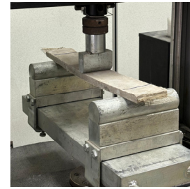
Fig. 4 Three-point bending test (a) schematic diagram; (b) experimental setup
