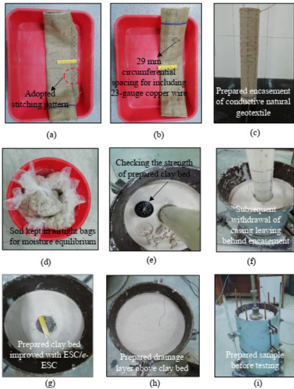
Fig. 3 Various components of the test procedure (a) adopted pattern for making encasement, (b) prepared encasement with a marking for inclusion of copper wire, (c) prepared encasement, (d) sample kept for moisture equilibrium, (e) confirming the strength of prepared clay bed, (f) preparation of column, (g) prepared clay bed improved with ESC/e-ESC, (h) prepared drainage layer and (i) prepared final sample
