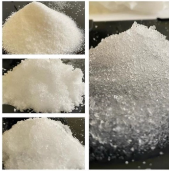
Fig. 2 A formation of gel structure due to water content increase in sodium polyacrylate powder (Güler 2022)
