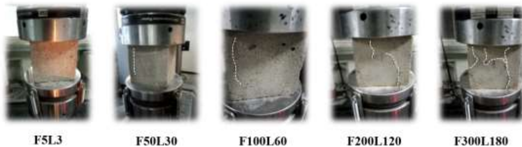
Fig. 8 Surface morphology of foamed concrete under cyclic loading
