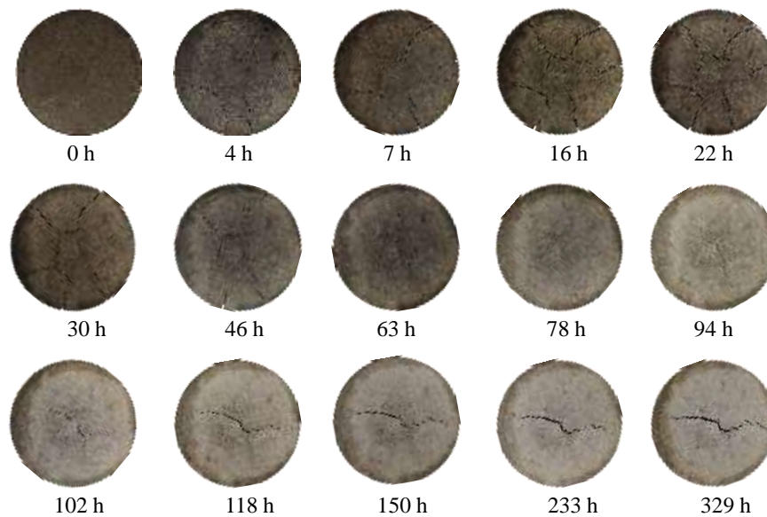
Fig. 6 Variation of fissures of compacted bentonite sample W35 with time
