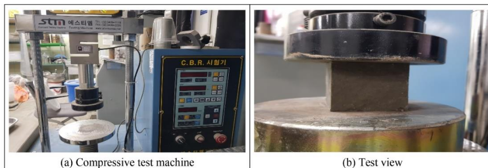
Fig. 3 Compressive test machine and test-view
