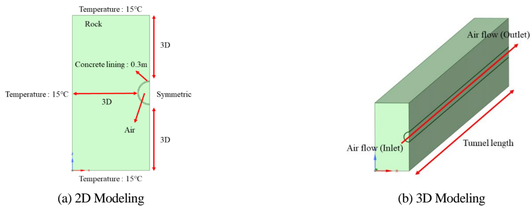
Fig. 4 Tunnel modeling and boundary conditions for model validation
