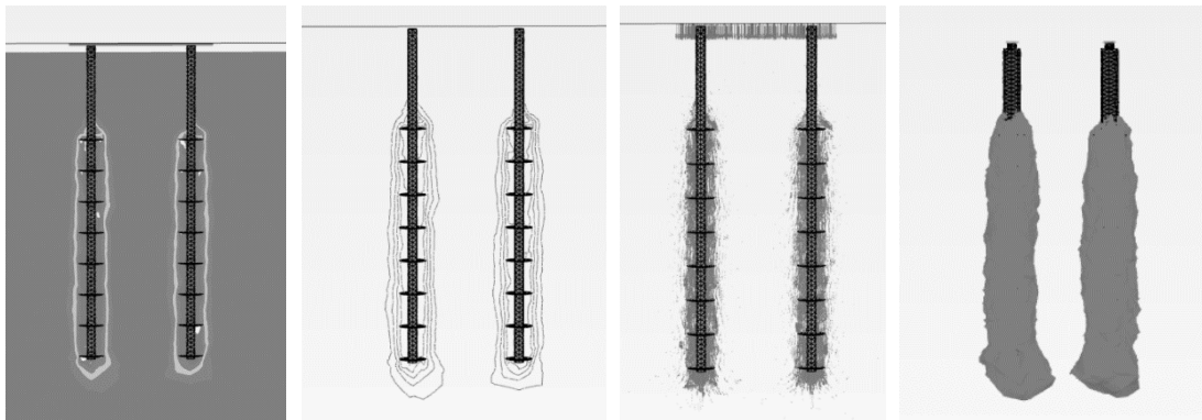
Fig. 12 Failure surfaces of screw piles under compressive force
