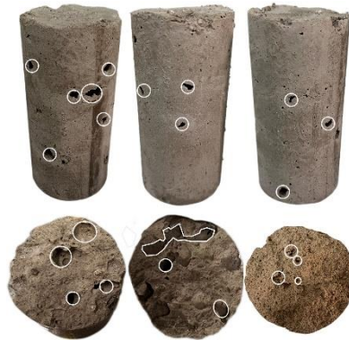
Fig. 5 Similar materials of CRL with prefabricated pores
