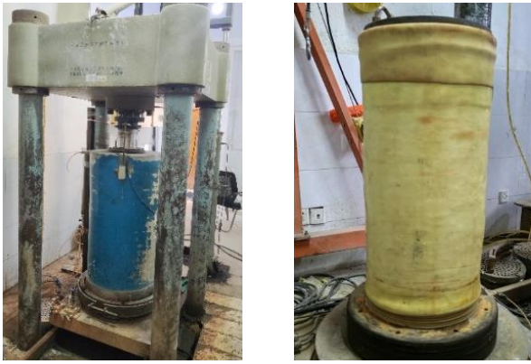
(a) Large-scale triaxial apparatus (b) Sample preparation apparatus
