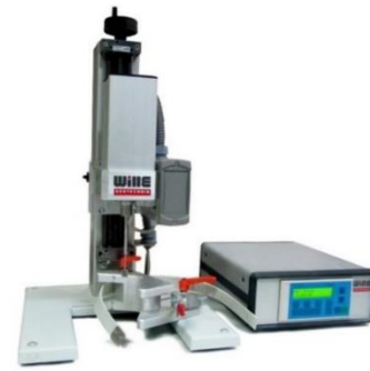
Fig. 3 Laboratory type Vane Shear Test (VST) device
