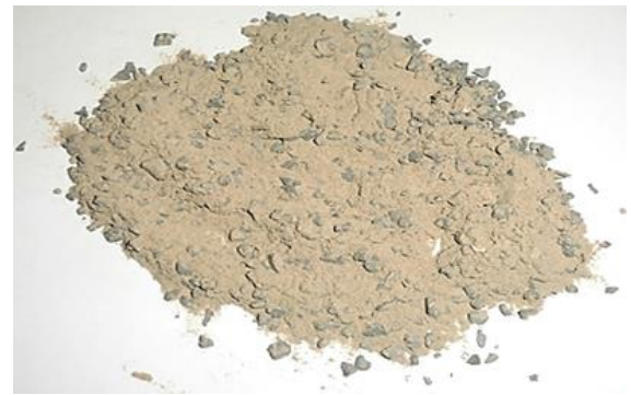
Fig. 3 PVC granules mixed with soil
