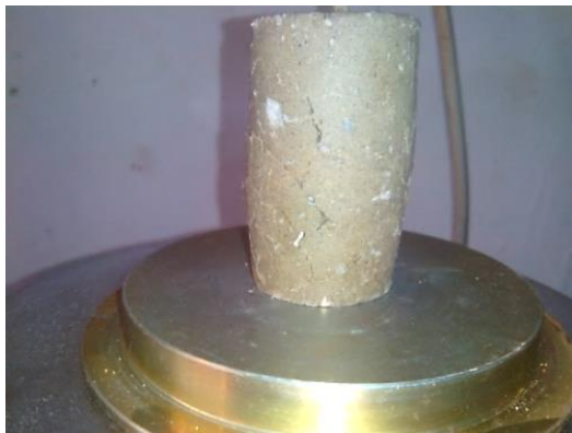
Fig. 5 The sample after compression testing
