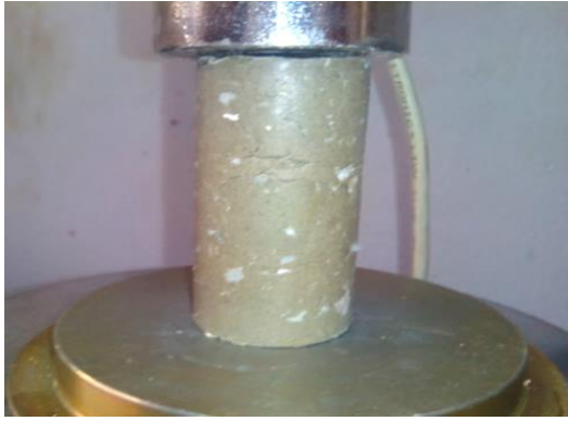
Fig. 4 Uniaxial compressive strength test
