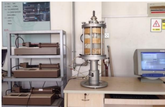
(a) The GDS stress path triaxial system
