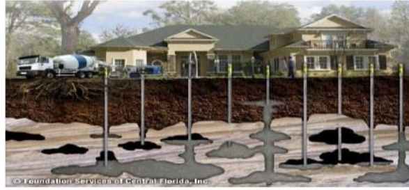
Fig. 2 Grouting for Sinkhole Remediation (Foundation Services of Central Florida Inc. 2015)
