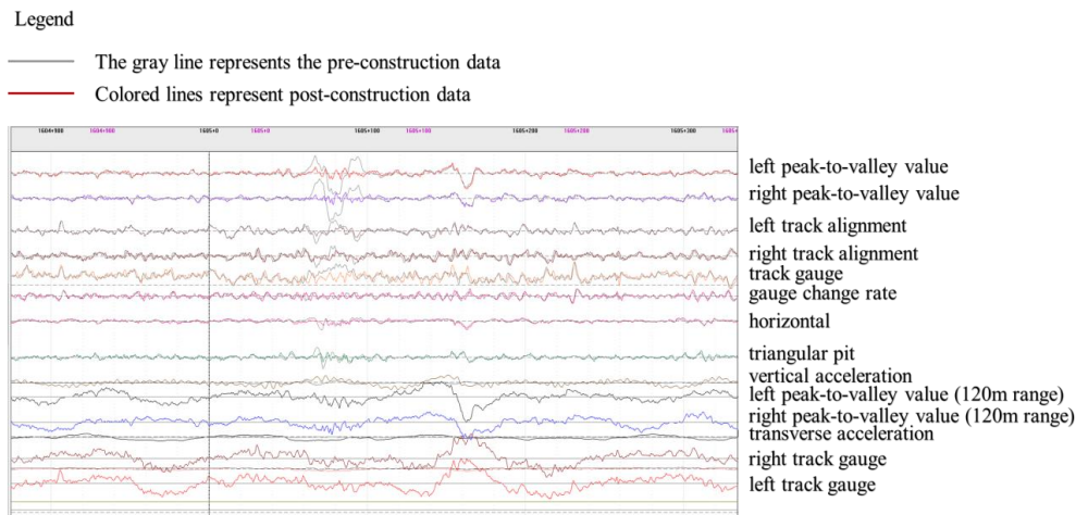
Fig. 16 Measurement results of dynamic inspection vehicle before and after construction
