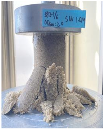
Fig. 1 Failure mode of sand treated by the MICP surface percolation method during UCS testing. The lower part crumbles first because there is less cementation than in the upper part.
