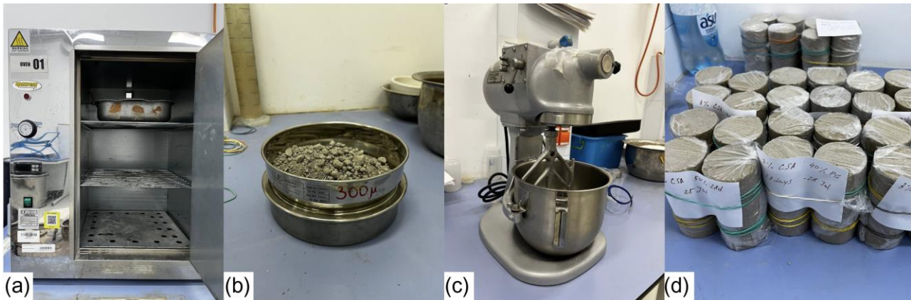
Fig. 4 Sample Preparation Process:(a) Drying of sand and PG for 24 hours; (b) Sieving of PG; (c) Mixing of materials and (d) Curing for 3, 7, 14, and 28 days
