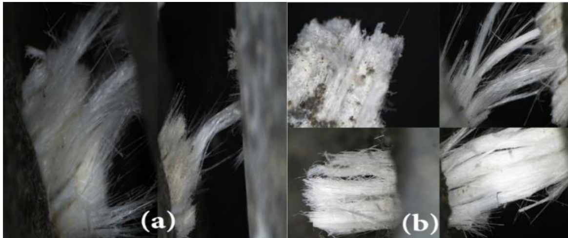
Fig. 14 Microscopic textile damaged spots: (a) 0.3G/370/L and (b) 0.4G/370/L
