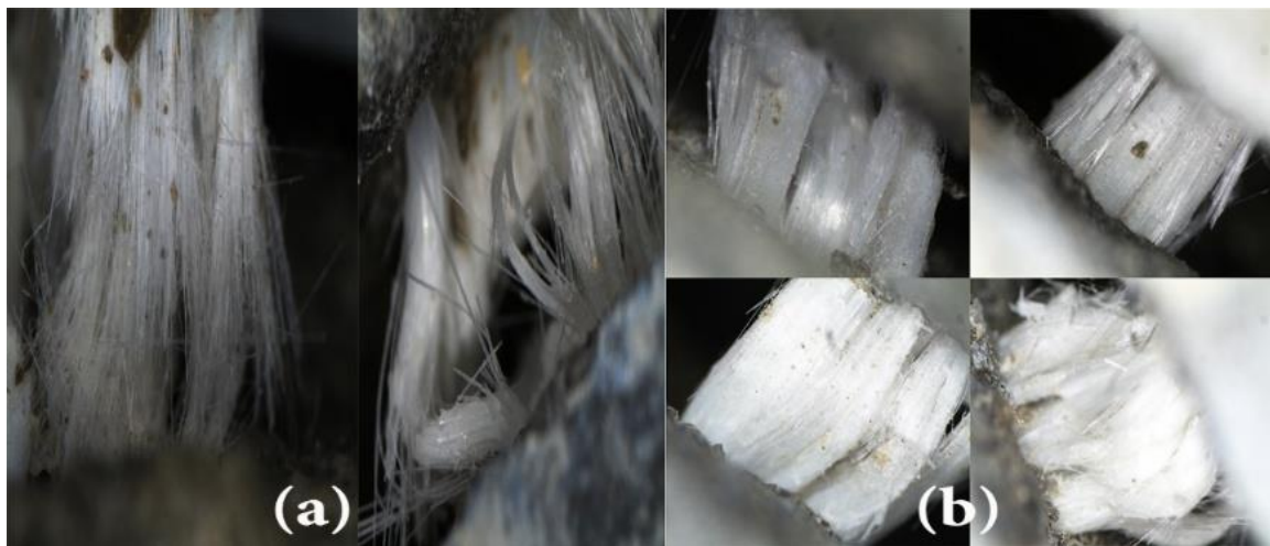
Fig. 12 Microscopic textile damaged spots: (a) 0.3G/680/L and (b) 0.4G/680/L
