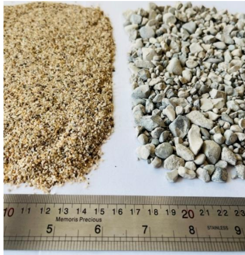
Fig. 1 Clean, medium-sized silica sand ( left photo ) used for preparing the medium-dense soil beds and well-graded SwG soil ( right photo ) used in forming the thin densified coarser layers incorporated within the sand beds
