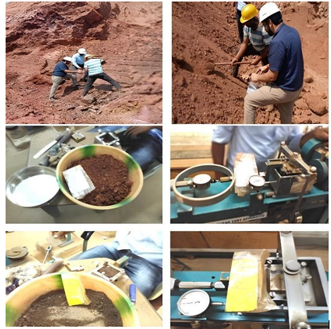
Fig. 6 The Collection & Preparation of Sample and Direct Shear Testing in the Laboratory
