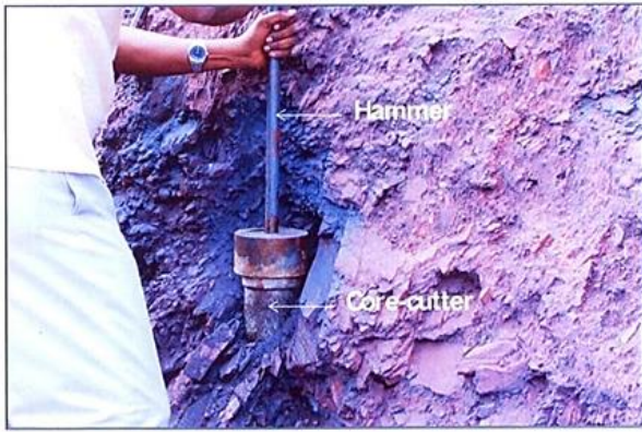
Fig. 4 In-situ bulk density determination and sample collection
