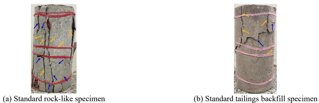
Fig. 6 Macroscopic failure mode of intact specimens
