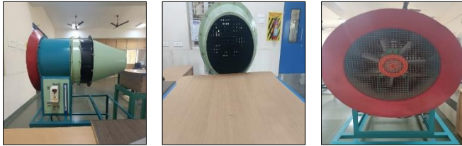
Fig. 3 (a) Wind tunnel, (b) airflow duct and (c) fan motor
