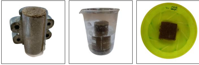
Fig. 2 (a) Cylindrical sample preparation for strength and immersion tests, (b) Jar immersion test and (c) Crumb dispersion test
