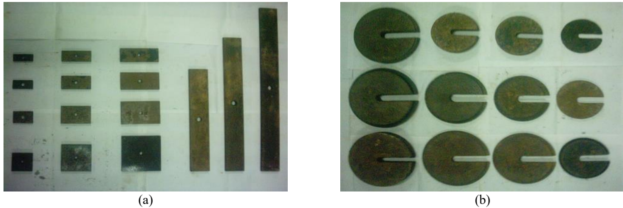
Fig. 2 (a) Different sizes of model anchor plates (b) Dead load used for the test and
