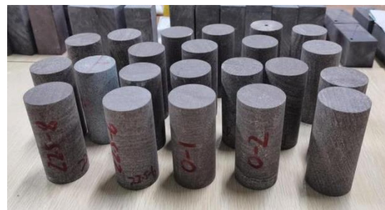
Fig. 2 Standard sandstone samples with different bedding dip angles
