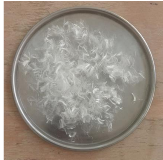
Fig. 4 Polypropylene fibre reinforcement used in this study
