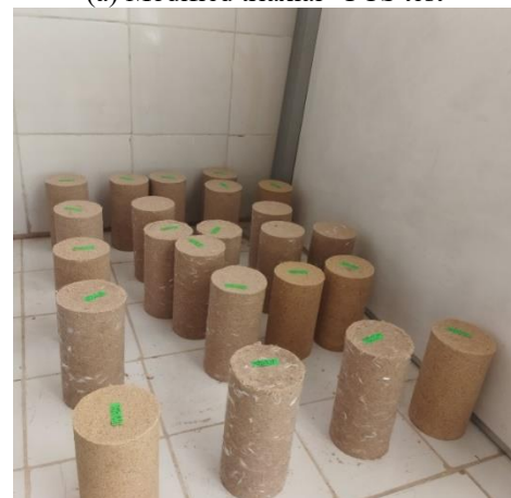
(b) Airing for curing samples
