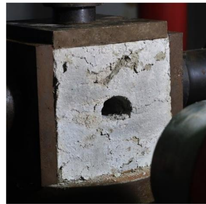
Fig. 4 Crack initiation in specimen 1#
