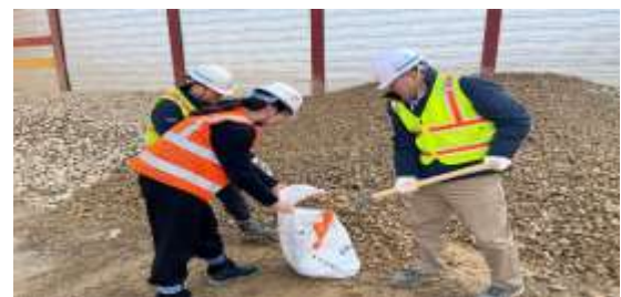
Fig. 5 Sample collection of filter cake and aggregate from filter press and slurry treatment plant
