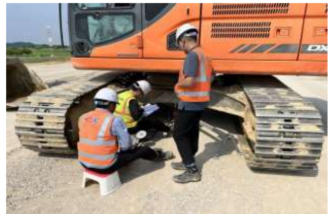
Fig. 6 Plate bearing test
