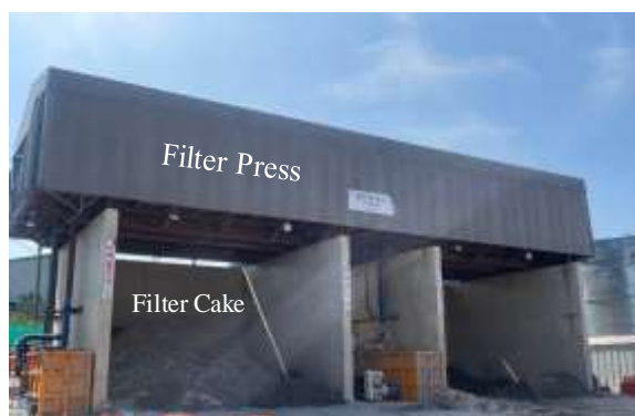
Fig. 4 Filter cake in filter press
