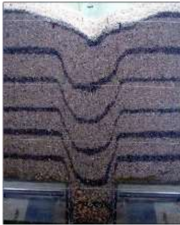
(a) Soil deformation
