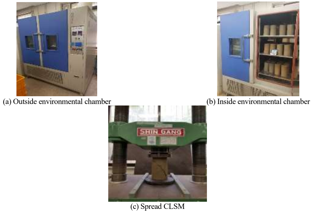
Fig. 5 Compressive strength tests: (a) outside the environmental chamber, (b) inside the environmental chamber, and (c) specimen after test completion
