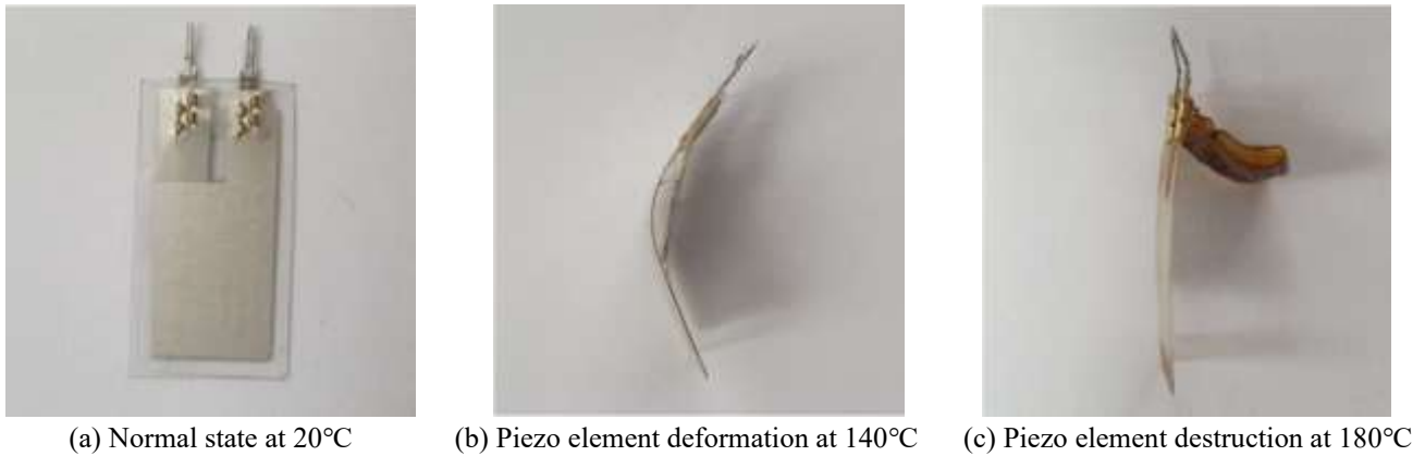
Fig. 7 Failure mechanism at different temperatures
