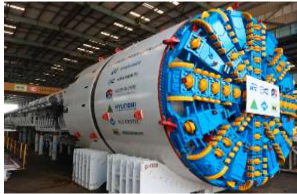
Fig. 3 Earth Pressure Balance Tunnel Boring Machine (EPB TBM).
