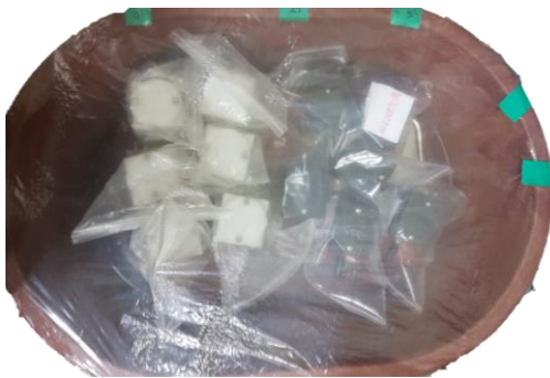
(d) Sealed curing chamber with small amount of water inside
