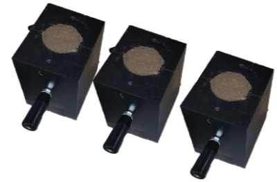
(c) Compacted specimens inside mold
