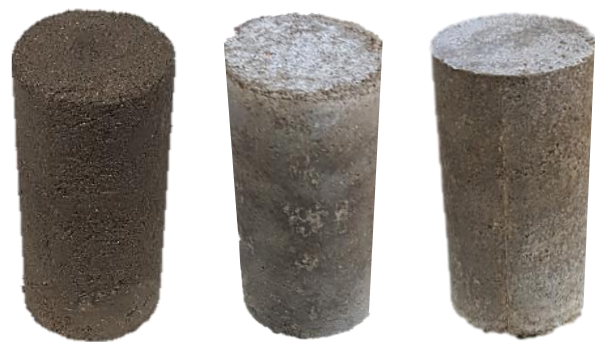
(e) Extracted specimens: 5% WA-WS, 15% WA-WS, and 25% WA-WS
