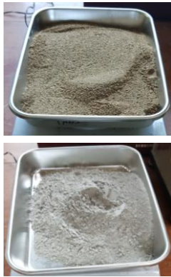
(a) Preparation of WS and WA portions: 5%, 15%, and 25% (by dry mass of soil)
