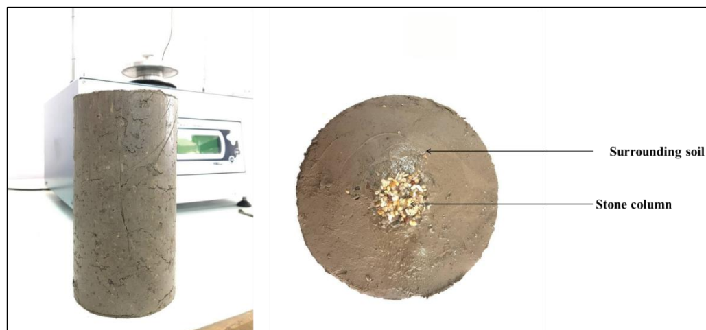
Fig. 4 Small model of stone column-soil in the triaxial cell
