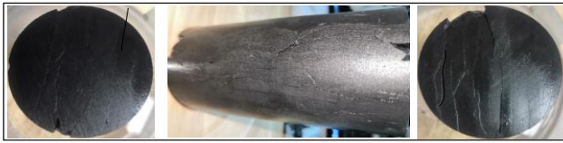
Fig. 8 Evolution of crack development in mudstone under soaking (Modified from Wu et al. 2020)
