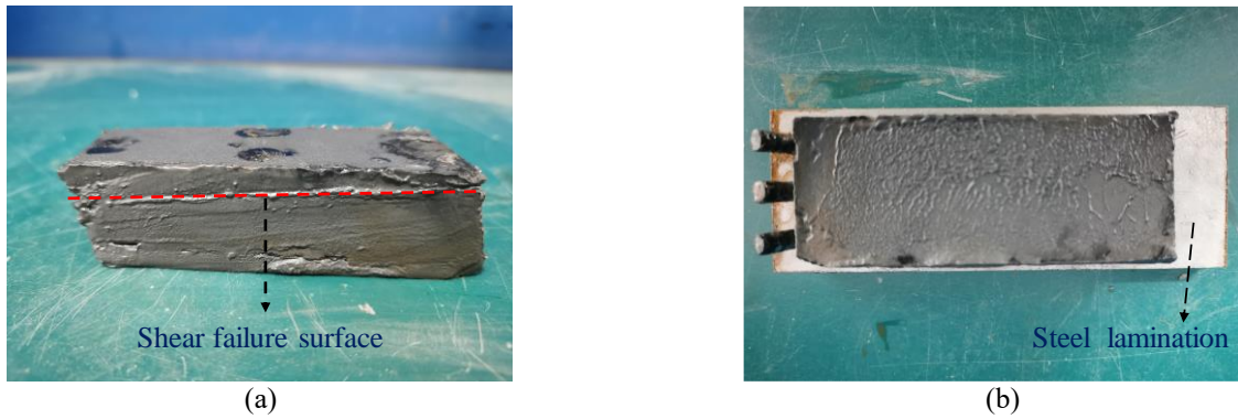
Fig. 9 Pictures of soil shear failure
