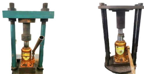
(a) Specimen making equipment (b) Specimen demolding equipment
