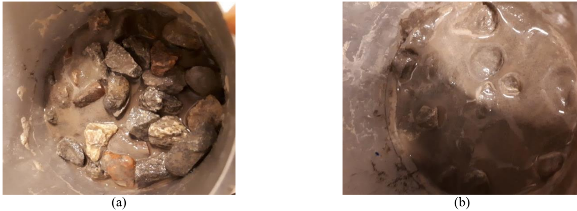
Fig. 8 Migration of tailings particles into the gravel layer (Ta_MoLCYC sample): (a) tailings particles at the top half of the gravel layer, and (b) tailings particles at the bottom half of the gravel layer
