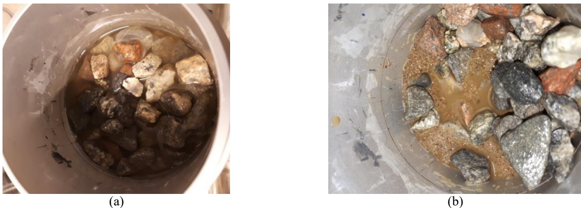
Fig. 11 Migration of sand particles into the gravel layer (RaSa_MoLCYC sample): (a) no sand particles at the top half of the gravel layer, and (b) sand particles at the bottom half of the gravel layer
