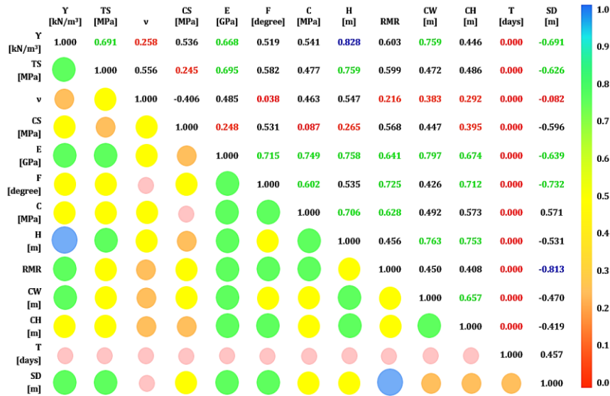
Fig. 3 The correlation matrix and relationships between input and output parameters affecting sidewall displacement
