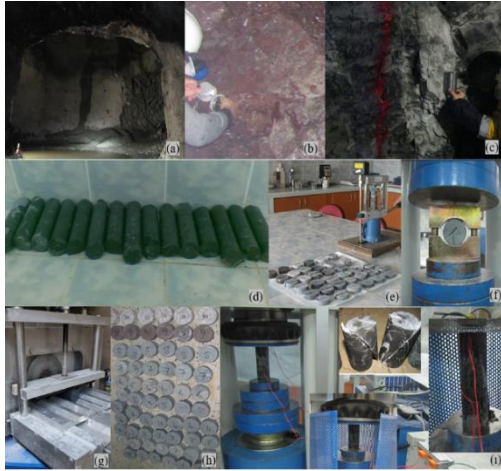
Fig. 3 Some examples of field and laboratory studies; a tunnel face (a), measurements of orientation by compass (b), measurements of roughness by profilometer (c), core samples from a tunnel face (d), PLI test (e), BTS test (f), core trimming (g) some samples for PLI and BTS (h) and UCS tests (i)
