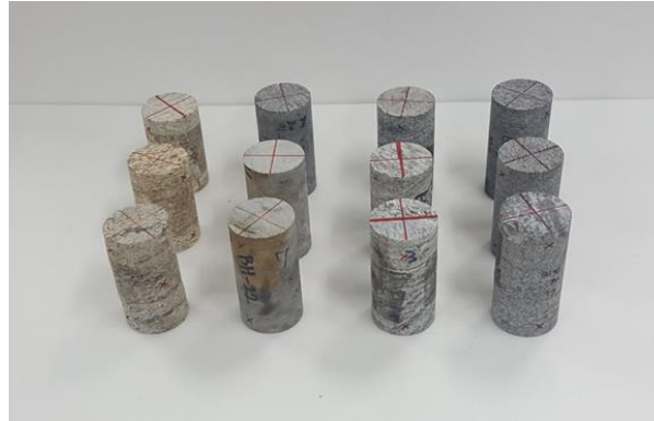
Fig. 1 Granite specimens for uniaxial compression test
