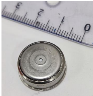
Fig. 7 Hygro-button photo and dimensions
