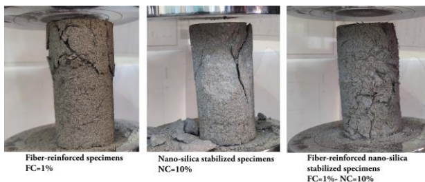
Fig. 7 Failure patterns of the specimens at the end of the UCS test
