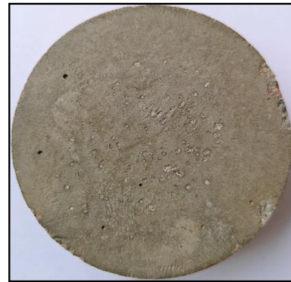
(b) Precast concrete-frozen soil interface
