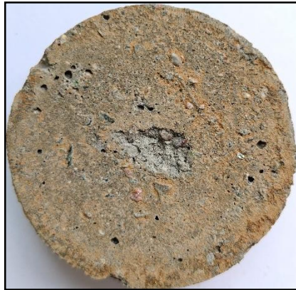
(a) Cast-in-place concrete-frozen soil interface
