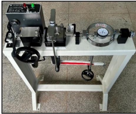
(a) ZJ strain controlled direct shear instrument
