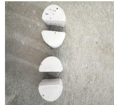
(c) After splitting test of analogue materials
