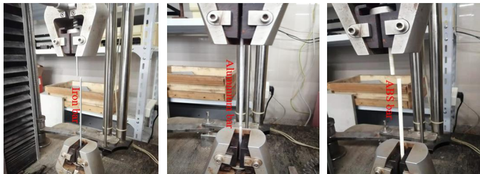
Fig. 6 Tensile damage diagram of the rockbolt materials
