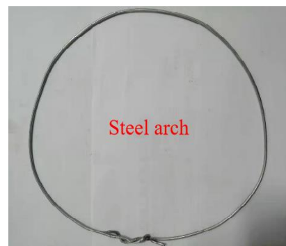
Fig. 16 Model of the steel arch
