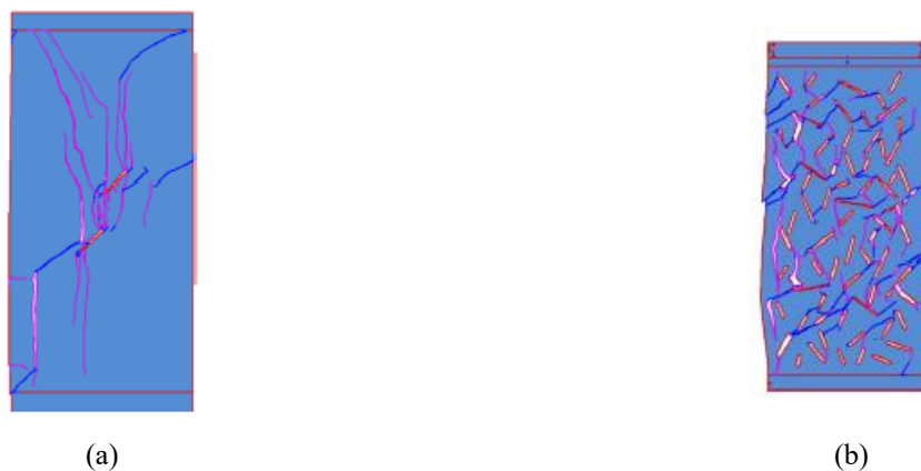
Fig. 35 All three modes of crack (I-tensile, II-shear, I-II mixed) captured using NMM for (a) double flaw and (b) Multiple random distributed flaws (after Kang et al. 2022)
