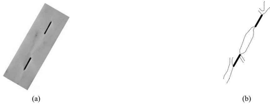
Fig. 16 (a) Development of white patch observed from SEM for marble specimen are 94% of failure stress and (b) Pattern of white patch shown in dotted lines (adopted from Wong and Einstein 2009c)
