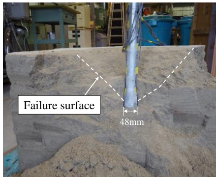
Fig. 7 The failure shape of the soft-rock ground after terminating the pull-out test of belled pile
