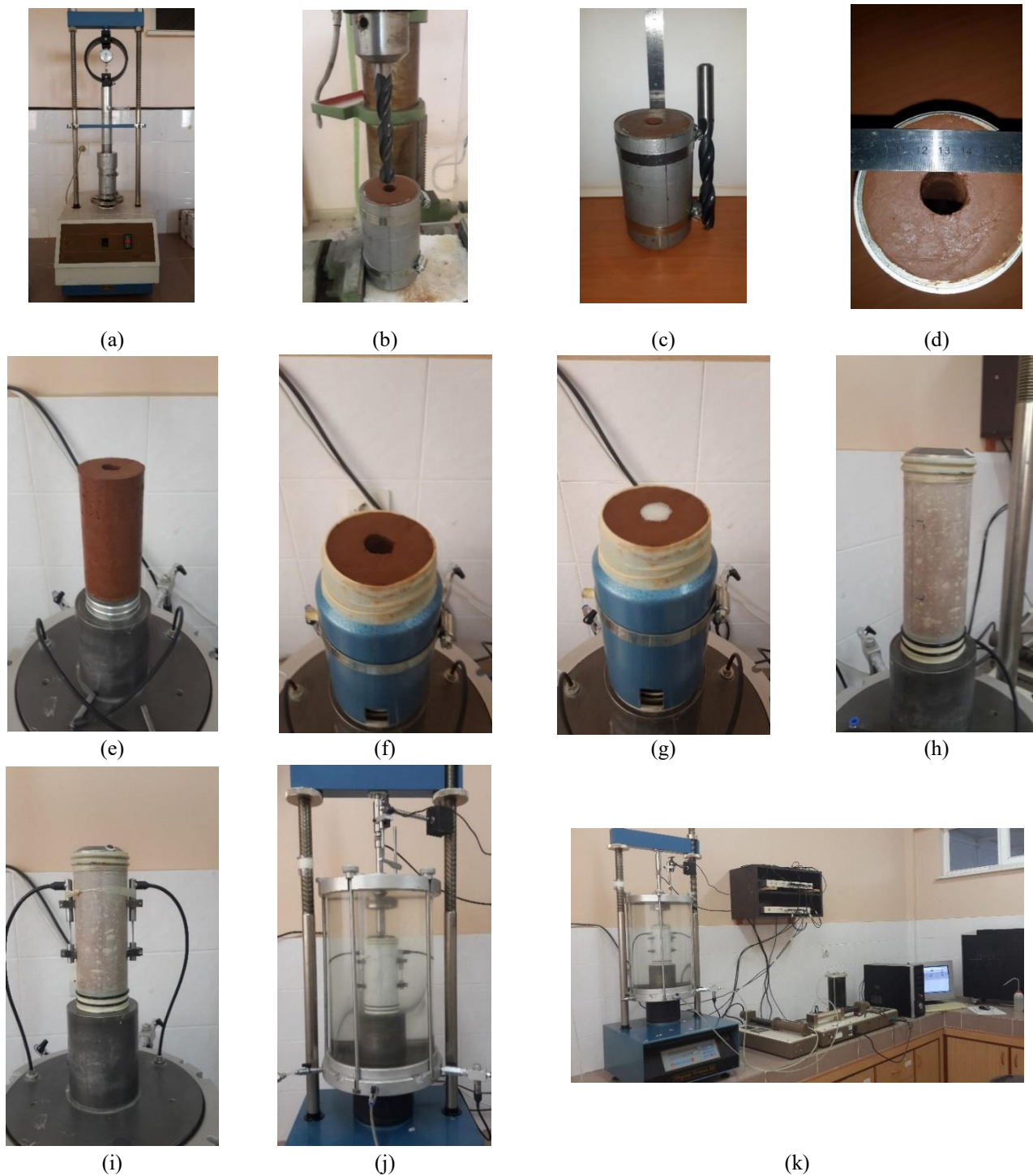
Fig. 5 Triaxial tests sand column specimen preparation processes
