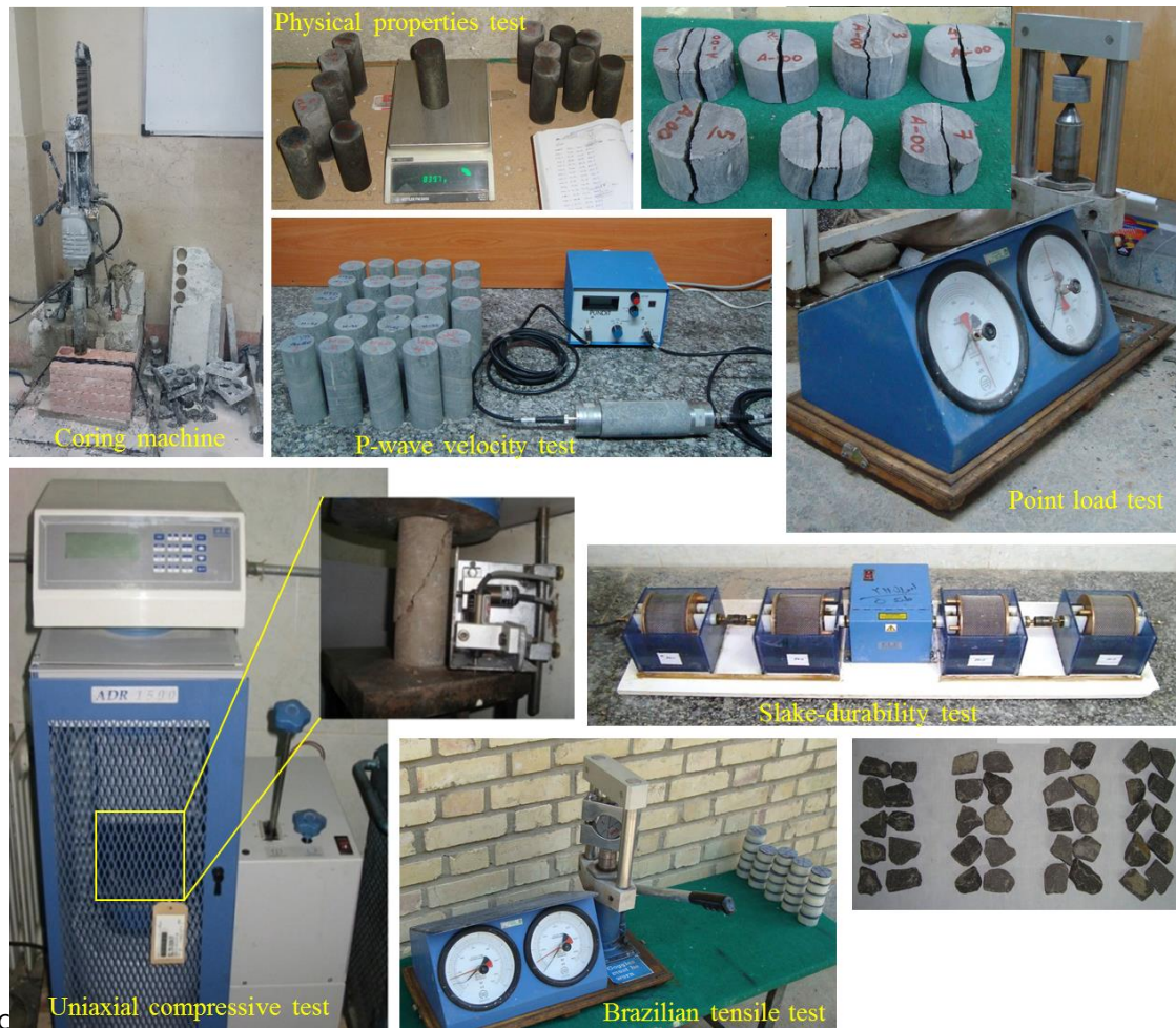
Fig. 3 Application of various laboratory tests on the studied rocks
