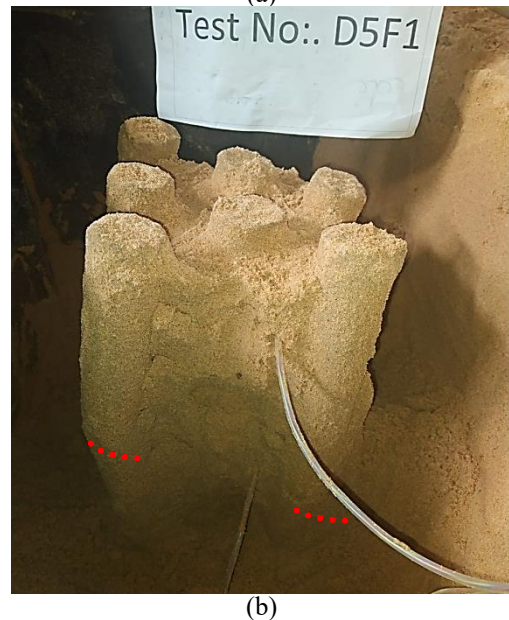
Fig. 16 Fracture of DSM columns at D5F1 test (a,b)
